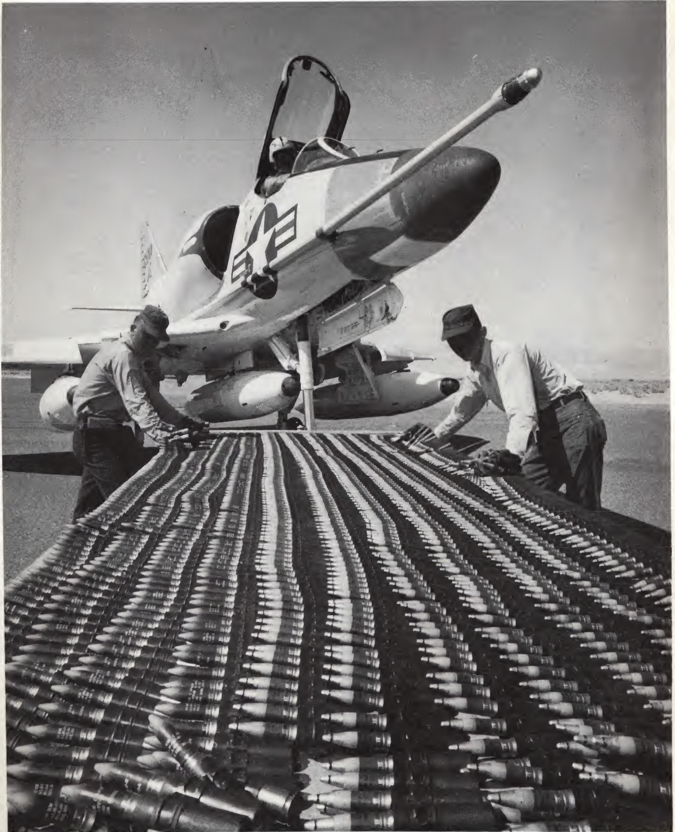
Figure 1-1. Three Gun Pods Mk 4 Mod 0 Installed on A4 Aircraft
